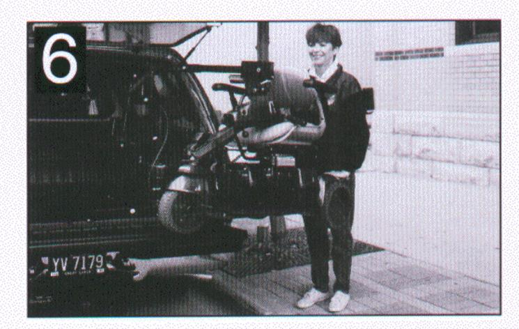
The Curb-Sider can also be used to raise and store a fully assembled scooter in vehicles with tailgates, so long as the opening is large enough to accommodate the lift and scooter.
