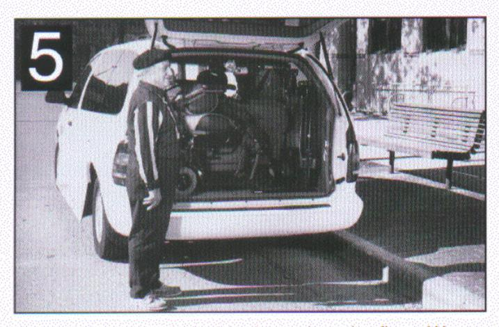
Once the scooter is inside, lower it to the floor. We recommend that you leave the C-arm attached to secure the scooter during travel.
